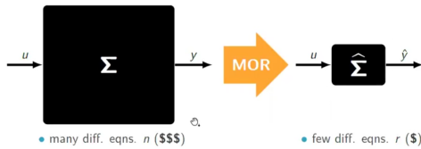
Fig. 1: Visualisation of basic concept of MOR. A large system \Sigma with described with many equations n can be reduced to a smaller system \hat{\Sigma} with many fewer equations r .
